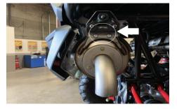
**3.** Remove the three bolts securing the hanger shield, then remove rubber insulator and then the shield. Next, remove the factory muffler by sliding it off the driver side hanger. Use WD-40 to lube the rubber insulators to aid removal.
