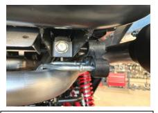
4. To install the Gibson muffler (Item A), re-install the factory rubber insulators on your new muffler assembly and install the muffler onto the factory hangers. Then install and tighten the flange bolts for the head pipe using Item G) included in the kit are shorter flange springs.
